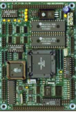
CPU: CMOS 68HC16Z1 with 16.78 MHz clock speed
