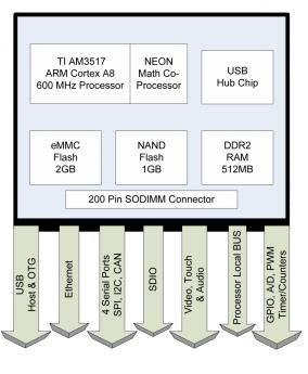
Using the same small 200 pin SODIMM form-factor utilized by other EMAC SoM modules, the SoM-3517M is the ideal processor engine for your next design. All of the ARM processor core is included on this tiny board including: Flash, Memory, Serial Ports, Ethernet, SPI, I2C, I2S Audio, CAN 2.0B, PWMs, Timer/Counters, A/D, digital I/O lines, video, Clock/Calendar, and more. The SoM-3517M additionally provides a math coprocessor, and 2D/3D accelerated video and image scaling/rotation.
