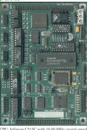
CPU: Infineon C515C with 10.00 MHz crystal speed, which has an internal equivalent clock of 20 MHz. Improved architecture results in 600 nS instruction cycle time at 10.00 MHz crystal speed.
