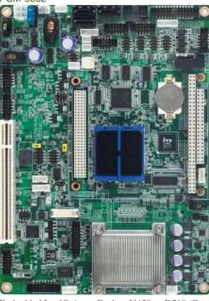
Embedded Intel® Atom Fanless N450 or D510 (Dual Core) Processor
