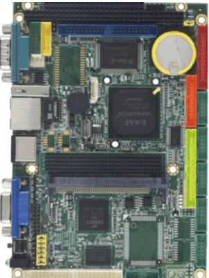
CPU: Fanless Vortex 486 class 86DX running at 800MHz
