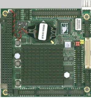
Onboard AMD Geode<sup>TM</sup> LX800 Processor
