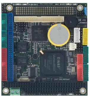
CPU: Fanless Vortex 486 class 86DX running at 800MHz
