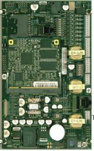
The SoM-250ES is a compact, low-power SoM Carrier/Socket board with a optional 7" WVGA (800 x 480)
