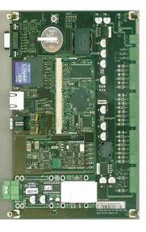
When a unique custom board is required for an application, the amount of design work required is greatly minimized by the SoM approach. The custom Carrier designer does not have to worry about the processor, memory, and standard I/O functions and can concentrate on the I/O, connectors and dimensional aspects required for the application.
